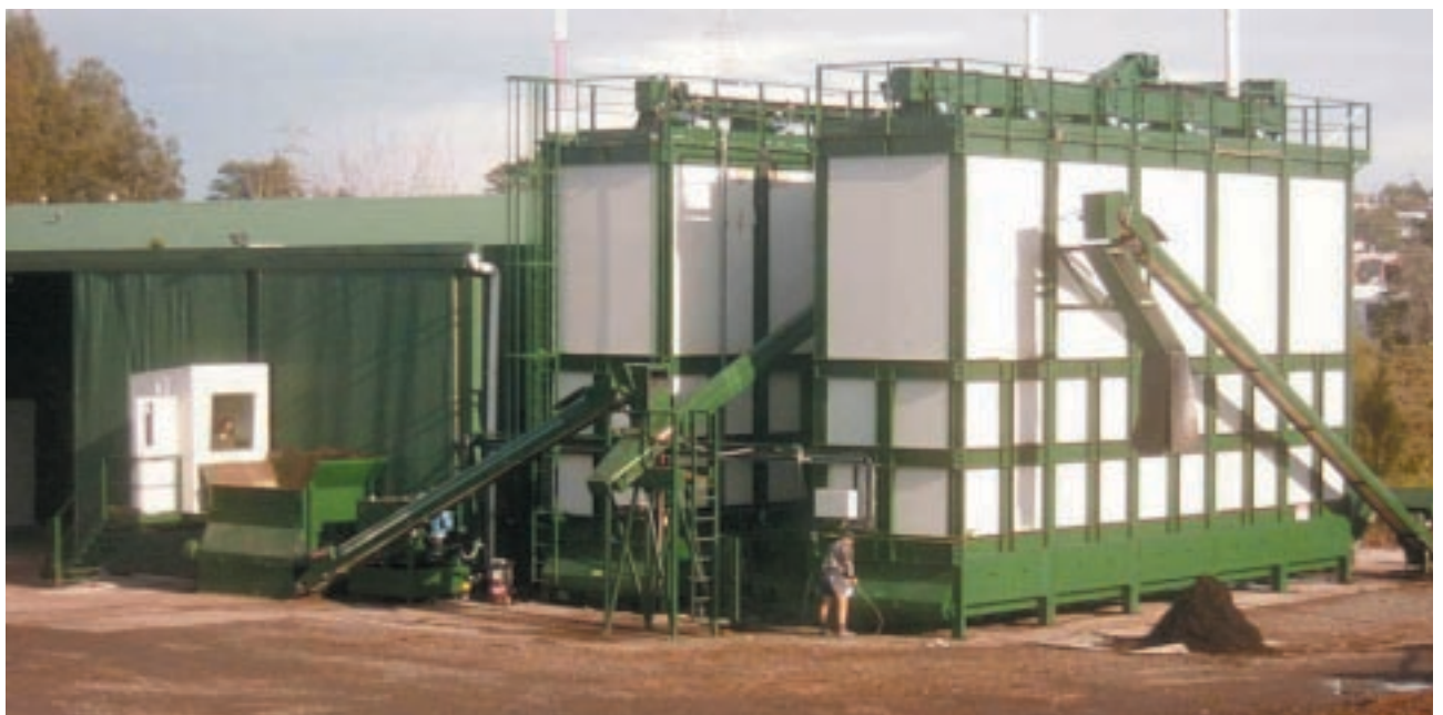
A Vertical Composting Unit. VCU sites in Australia and New Zealand process a wide range of organic materials – including green waste, food processing wastes, paper and sewage sludge.
